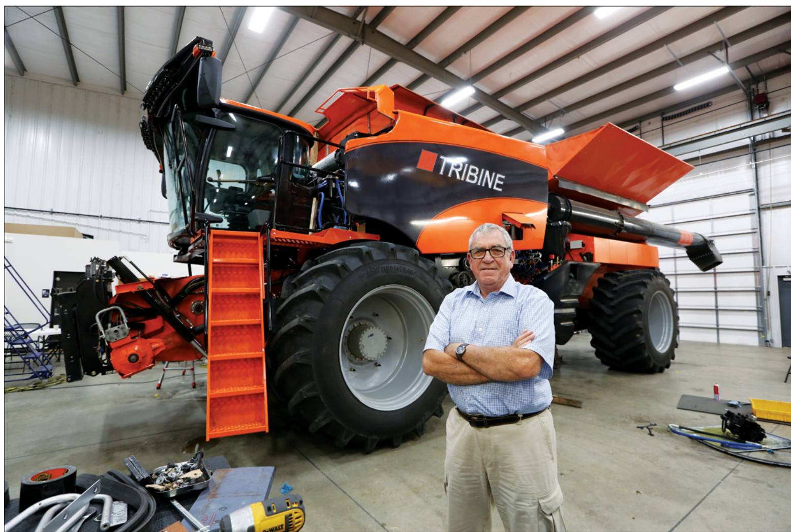
Ben Dillon stands next to his innovation in harvesting technology at the Tribine Harvester complex in Newton on Aug. 4. Dillon's invention puts a combine and a 1,000-bushel grain tank together into one machine.
